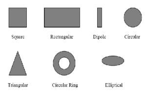
Fig. 3. Some shapes of microstrip patch elements.
