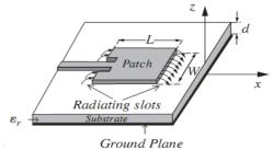
**Fig. 4.** Fringing Filed between the Patch and the Ground Plane.
